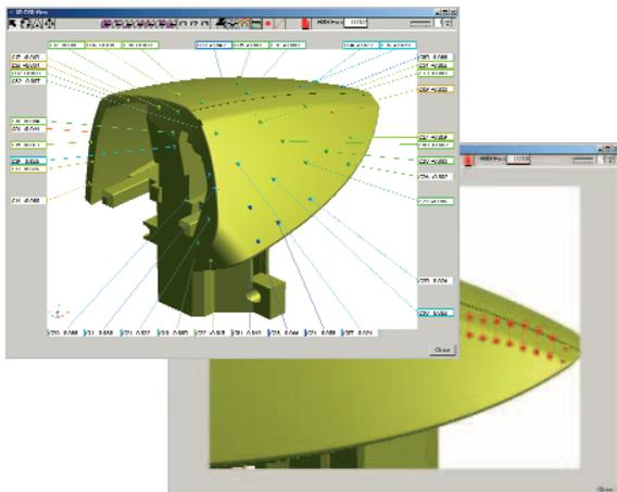
The best-fit function allows full 3D re-alignment of the model in order to minimise the RMS errors of any set of measured points within a curve unit.
