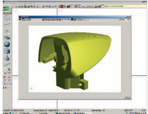
The solid model appears in an additional floating window on top of the main Aberlink 3D screen.
