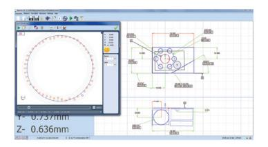
Aberlink 3D software is revolutionary. As a component is measured a representation of it is built up on the screen. The user simply clicks on the measured features to call up dimensions exactly as they would appear on a drawing.
